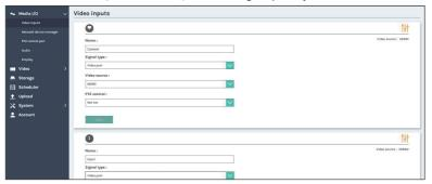
While assigning the "network camera" as the [Video source], an authentication process from the camera may be needed in [Network device manager] setting up tab of [Media I/O].
